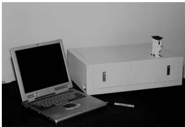
Fig. 10. Appearance of the portable dichrometer designed for the solution of analytical problems using biosensors based on the DNA LCD.
